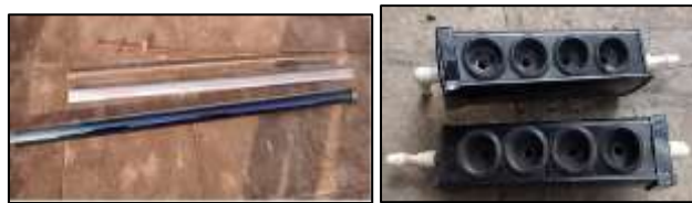
Fig.6- Heat Pipe, Evacuated Tube, Aluminium strip and Insulated Manifold of condenser section guide.
